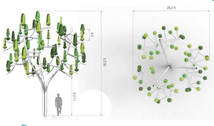
The WindTree is a steel structure (trunk and branches) on which 54 Aeroleaf® are installed.
