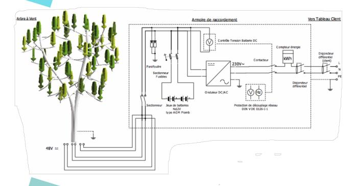
The Windtree is connected to the local grid through the Right Renewable Tech elected dedicated space should be prepared for the cabinet, within a maximum distance of 50 meters.
